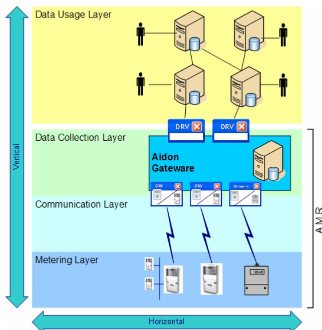
Fig. 2. Aidon AMR – openness driven solution.
